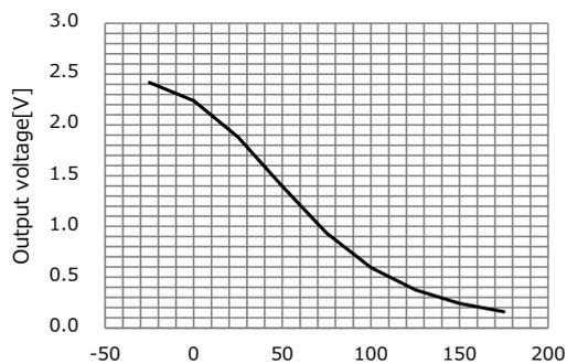
IGBT thermistor temperature[°C]
