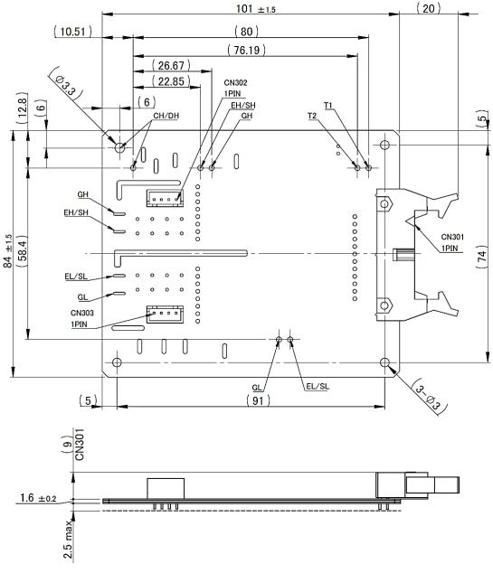
Unit: mm Note: 1. The dimensional tolerance without directions is  $\pm$  0.5mm.
