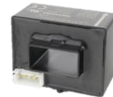
(b) NEW ASIC current sensor LA37S200S05
