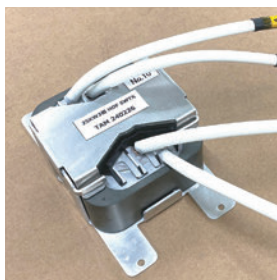
HDF switching transformer
