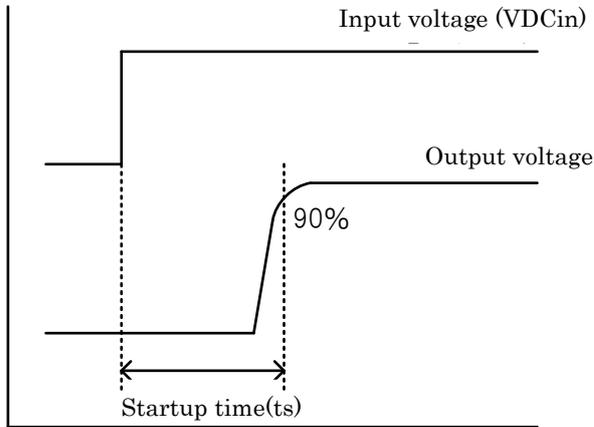
The startup time can be adjusted by connecting an external resistor and capacitor as follows:
