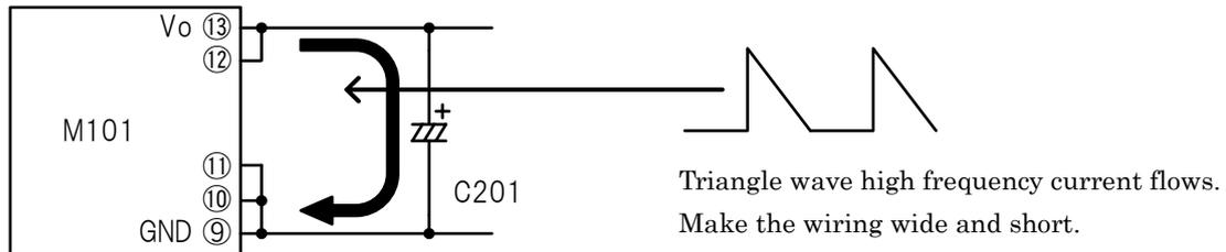
② Use an electrolytic capacitor with good frequency characteristics and low impedance.
