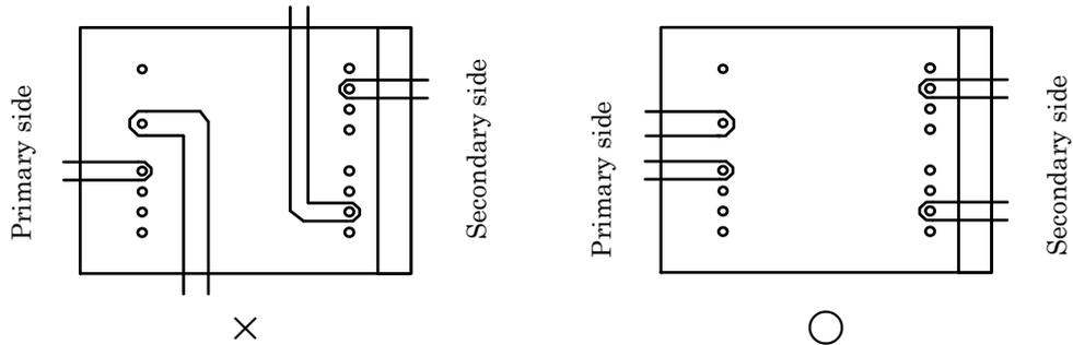
The installation prohibited area of primary parts and secondary parts is shown in the figure below. Do not install parts inside the dotted lines.
