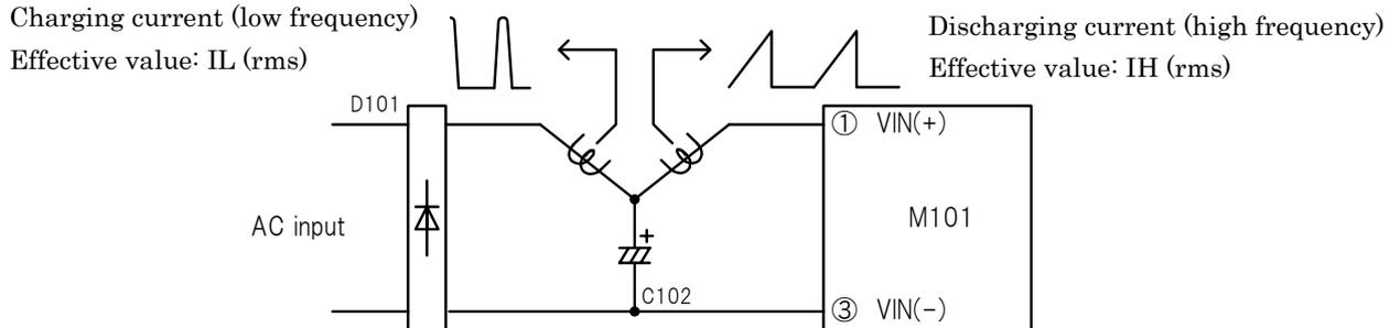
The ripple current ( $I_{120}$ ) frequency corrected to 120Hz is calculated from the following expression:
