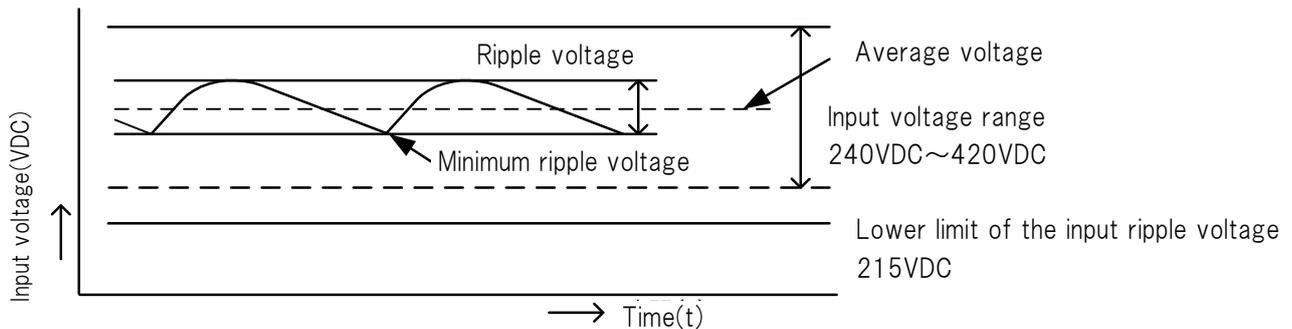
The capacitance of the electrolytic capacitors can be estimated using the formulae below.
