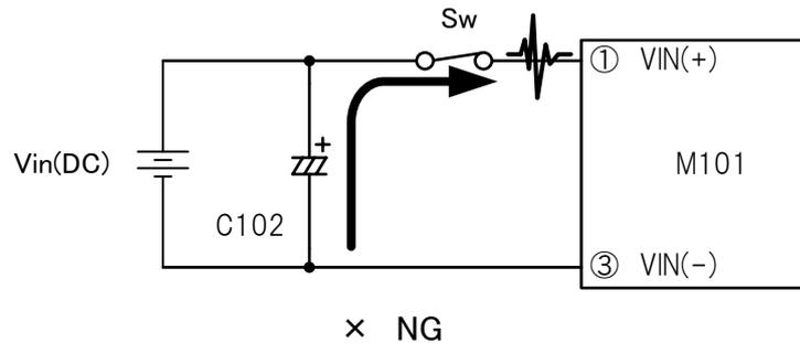
① Install the capacitor very close to the module (M101) and use a wide pattern to connect M101.
