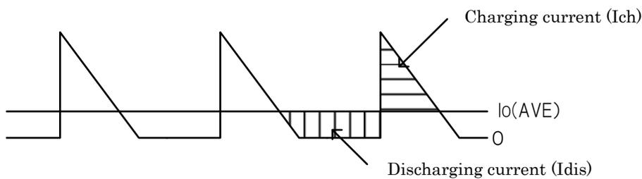
$$I_{ripple} = \sqrt{I_{dis}^2 + I_{ch}^2}$$
