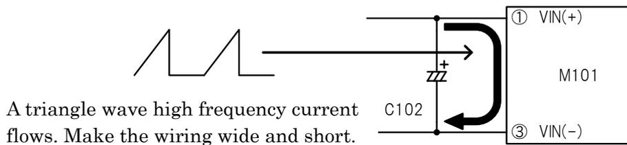
② Follow the instructions below to determine the capacitance of the electrolytic capacitors according to the input voltage to be used.
