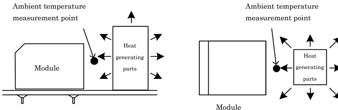
Ambient temperature measurement point when there is no effect of heating generating part
