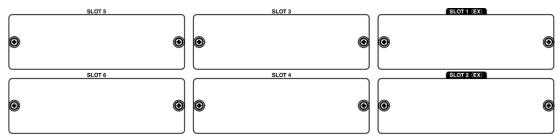
Insert optional IO CARDs of various types to these slots. IO CARDs of different types can be inserted to the slots.
