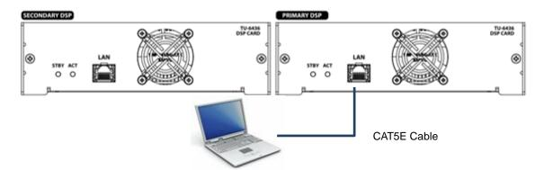
[Connection with a computer: Two DSP CARD configuration Secondary DSP CARD = ACT]
