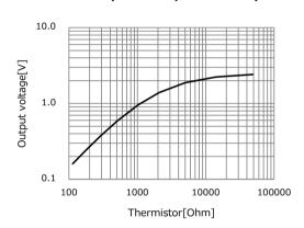
Thermistor signal output voltage vs thermistor resistance value
