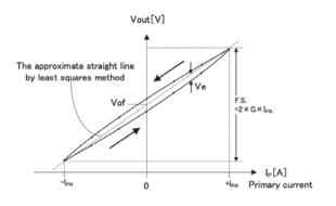
Sensitivity G[mV/A],Offset voltage Vof[V]
