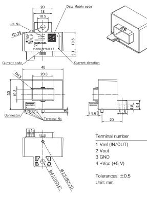
· Recommended fastening screw type : M4 with flat washer and spring washer  $\cdot$  Recommended fastening torque : < 1.5 N  $\cdot$  m
