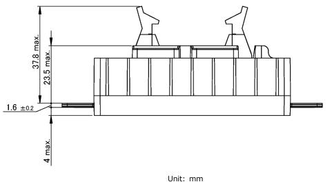
Note: 1. The dimensional tolerance without directions is  $\pm$  0.5mm.
