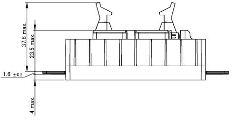
Unit: mm Note: 1. The dimensional tolerance without directions is  $\pm$  0.5mm.
