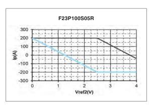
$$\begin{split} \text{Upper limit : lp = 200} & \text{(Vref2 = 0...2.5V)} \\ \text{lp = -160 \times Vref2 + 600} & \text{(Vref2 = 2.5...4V)} \\ \text{Lower limit : lp = -160 \times Vref2 + 200} & \text{(Vref2 = 0...2.5V)} \\ \text{lp = -200} & \text{(Vref2 = 2.5...4V)} \end{split}$$
