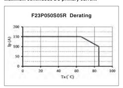
Figure 3: Ip vs Ta for F23P050S05R
