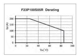
Figure 4: Ip vs Ta for F23P100S05R Measurement condition Vcc=+5V ,  $RL=10k\Omega$
