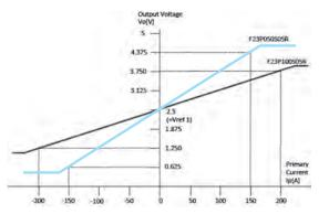
Figure 1 : Linearity curve (Internal reference voltage) Measurement condition Ta=+25°C, RL=10k $\Omega$ , Vcc=+5V
