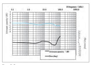
Figure 2 : Frequency response curve ex) F23P100S05R Measurement condition Ta=+25°C, RL=1k $\Omega$ , Ip=3A × 3T, Vcc=+5V
