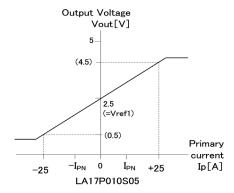
Fig 1 : Linearity curve Internal reference voltage)
