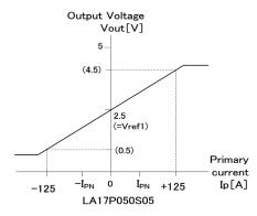
Fig 2 : Linearity curve Internal reference voltage)
