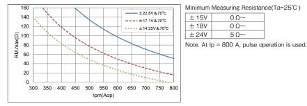
Fig1. Maximum Measuring Resistance  $\,({\rm Ta=70^\circ\!C}\,)$
